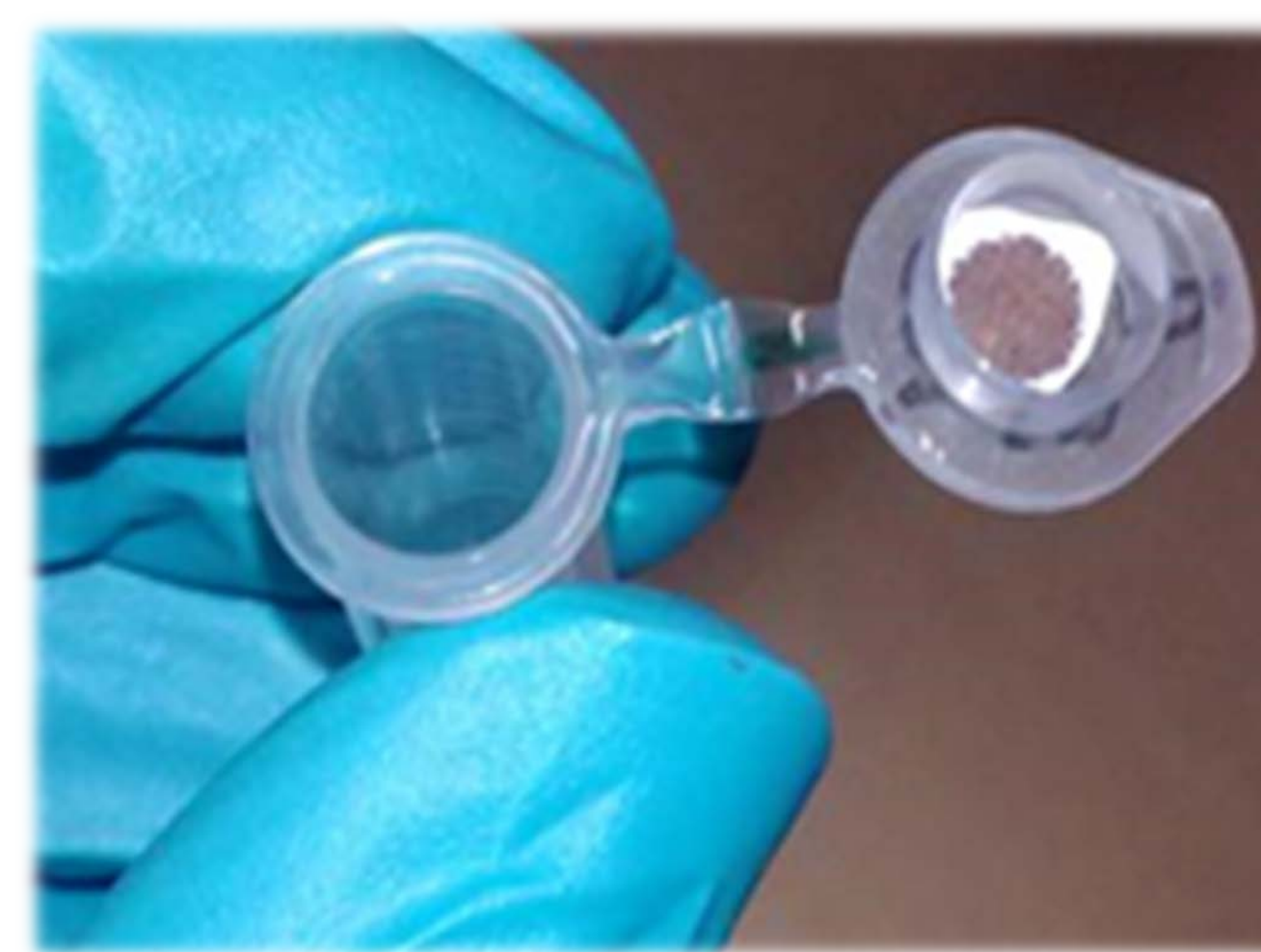
Figure 4: Dried samples placed in cap of 2 mL Eppendorf tube
