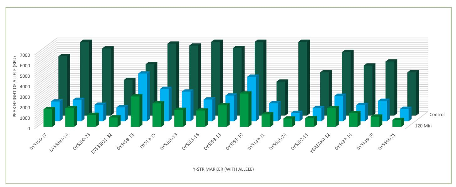
Artificial UV Exposure (254 NM): Y-STR markers (labeled on the X-axis) show significant loss of peak height (Y-axis) over the two hour time period (120 Min) of exposure when compared to the control sample which did not receive any sort of UV treatment and was stored in a dark room
