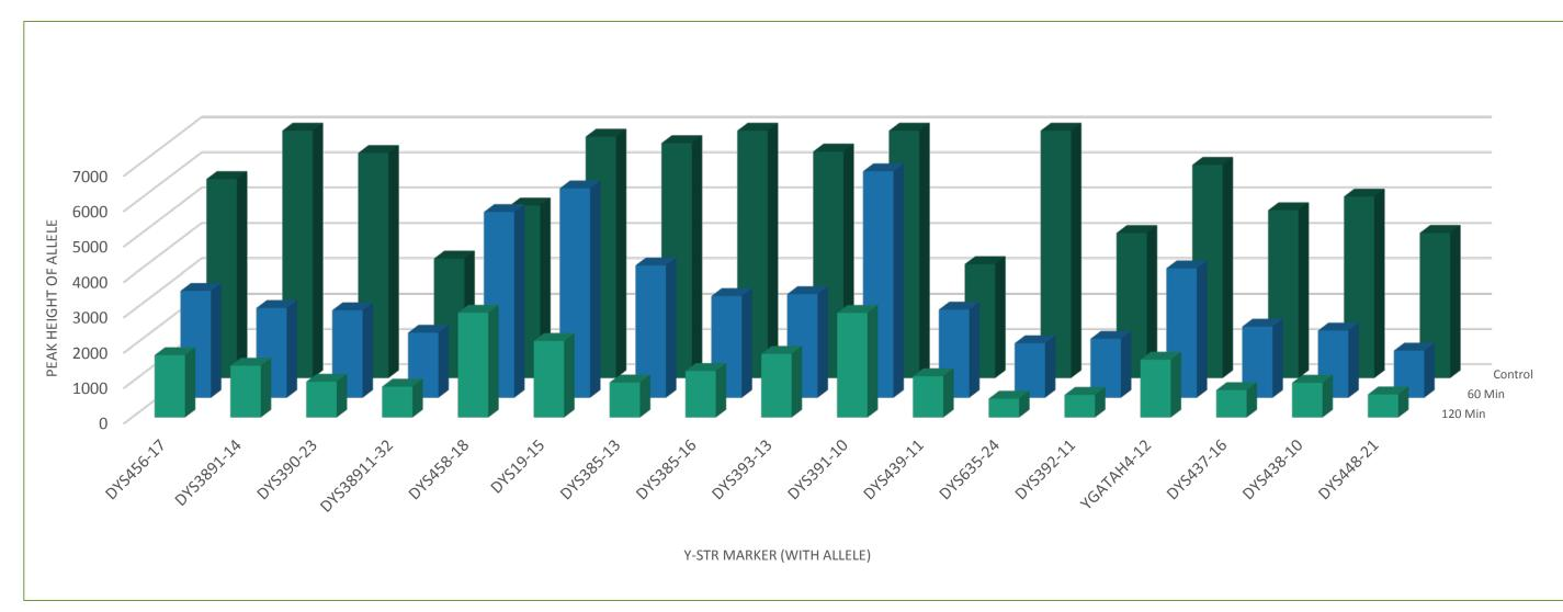
Artificial UV Exposure (302 nm): Y-STR markers (labeled on X-axis) show a significant decrease in peak height between the control samples (0 min) and the two hour (120 min) samples after exposure. One of the highest degrees of degradation can be seen in DYS635 marker that is greatly depleted after exposure.
